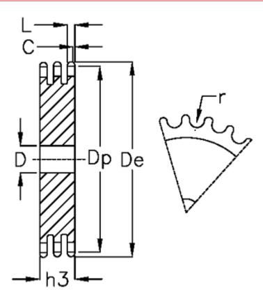
C = 1 D = 20 De = 161.8 Dp = 157.75 For chain size =  $3/8 \times 7/32$ For chain type = 06 B-3 h3 = 25.6
